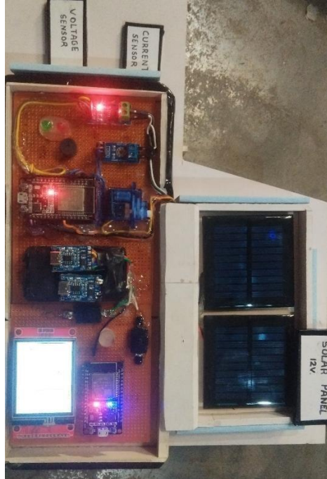
Fig. 4: Physical prototype hardware assembly of the smart solar energy monitoring and control system.
