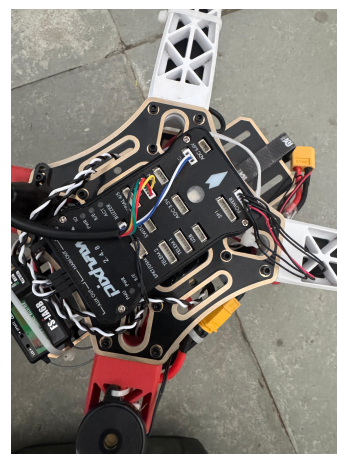
Fig. 3. Onboard Hardware Components Including Pixhawk Controller and GPS Module
