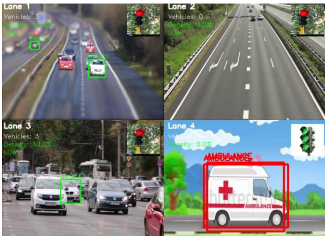
Fig. 9. Real time emergency vehicle detection
