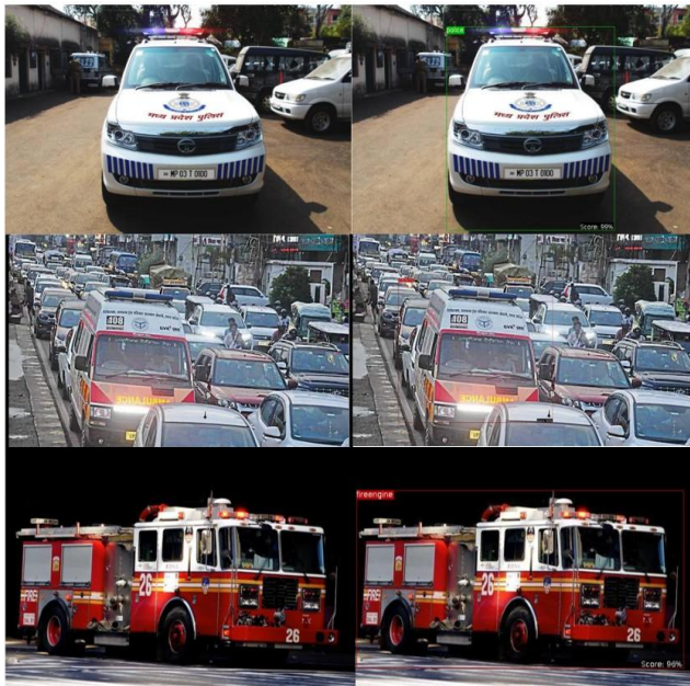
Fig. 5. The left figure shows the original image, while the image on the right side shows correctly identified emergency vehicles in boxes with class labels. Three classes of vehicle are identified: police, ambulance and fire engine.
