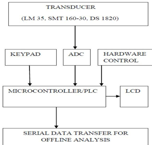
**Figure 1: Block Diagram for Experimental Setup [9]**
