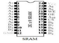
Figure1. Pin Diagram of SRAM
