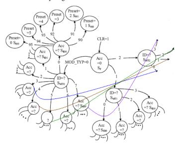
Figure3. Preset logic as FSM
