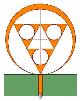
Fig No.3 Schematic of Proposed Sierpinski Gasket Antenna
