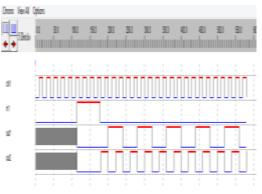
Fig.2:2-Bit Synchronous Up Counter
