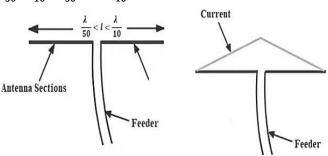
Fig 3d: Short Dipole Antenna (left) and Current Distribution in a Short Dipole Antenna [16]
