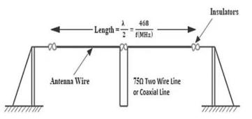
Fig 2: 1 MHz Dipole Antenna Design [16]
