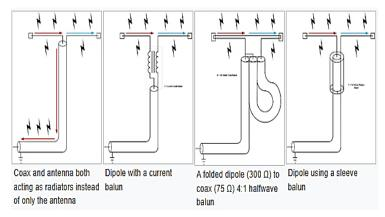
Fig6: Feeding a dipole antenna with coax cable[18]
