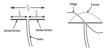
Fig3c: Basic half wave dipole antenna (left) and I and V distribution in a half-wave dipole antenna [16]
