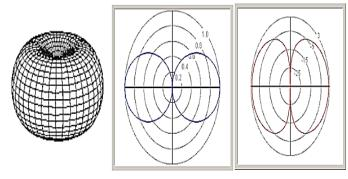
Fig5: 3D radiation pattern of a vertical half-wave dipole antenna (left); Radiation pattern of vertical half-wave dipole; vertical section (center) In linear scale (right) In decibels isotropic (dBi) [20]
