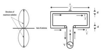
Fig1: Basic dipole antenna and its movement [16]
