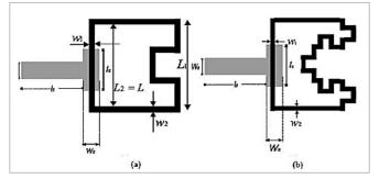
Fig 4(b): Antenna design with 1st and 2nd iteration fractal [23]
