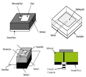
Fig 3: Microstrip Feeds: (a) Line feed (upper left); (b)proximity-coupling (upper right); (c) Aperture-coupling feed (lower left); and (d) Co-axial Feed (lower rt) [21]
