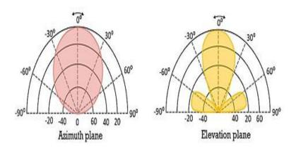
Fig 2: Radiation patterns of Microstrip Patch Antenna [16]
