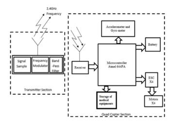
Fig. 1 Block diagram of the proposed drone system
