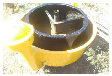
Fig6; Digester Inner side
