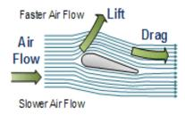
The pressure at the lower surface is greater and thus acts to "lift" the blade upwards, so we want to make this force as big as possible. When the blades are attached to a central rotational axis, like a wind turbine rotor, this lift is translated into a rotational motion.
