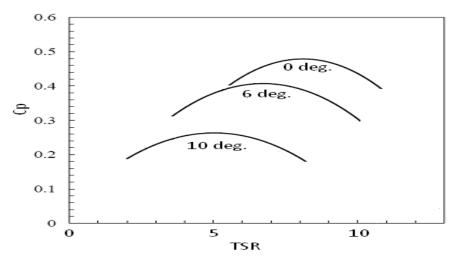
Fig.-Power coefficient Vs Tip Speed Ratio with Angle Of Attack.
