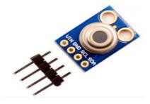
Figure 5.9 MLX90614 Temperature Sensor
