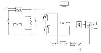
Fig 6. Simulink block for constant current mode
