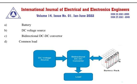
Fig.5 Converter and Battery Arrangement
