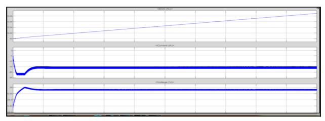
Fig. 13. . Simulink output - current flows from source to load when source enabled and battery charging
