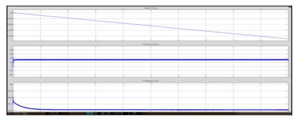
Fig.14. Simulink output - current flows from battery to load when source disabled and battery discharging
