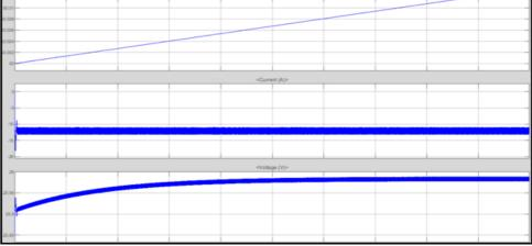
Fig.9. Simulink output - charging state of the battery at constant current mode
