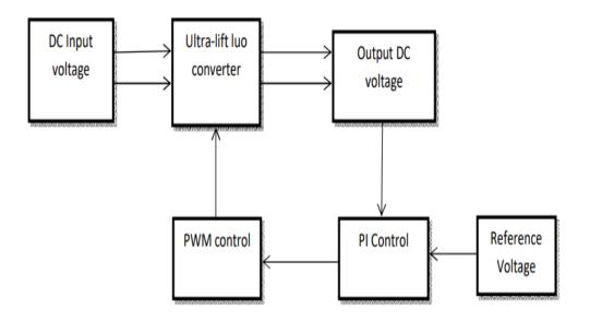
The DC input voltage is the power system voltage that uses only one polarity of voltage or current and have the constant, zero frequency which is applied to the Ultra-lift luo converter. Ultra-left luo converter is a type of converter which boost up the voltage level by reducing the ripple content from the DC voltage.
