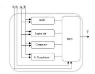
Fig. 1. Internal architecture of ALU
