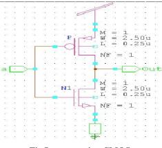
Fig Inverter using CMOS
