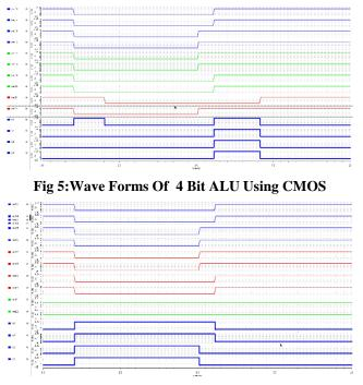
Fig 6: Wave forms of 4 bit ALU using GDI
