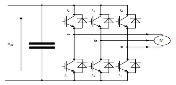
Fig 1. Three phase VSI using MOSFETs
