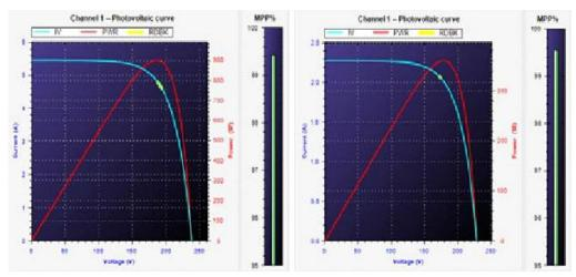
Fig. 6 (a) (b) MPPT performance at (a)  $1000 \text{ W/m}^2$ , (b)  $400 \text{ W/m}^2$
