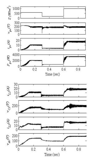
Fig. 5 Dynamic performances of the proposed SPV array based Zeta converter fed BLDC motor drive for water pump (a) SPV array variables, (b) Zeta converter variables
