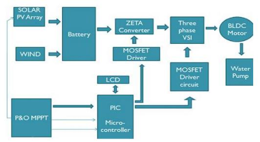
Fig. 2 ZETA Converter based BLDC motor driven water pumping system.
