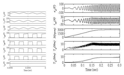
Fig.4 Starting and steady state performances of the proposed SPV array based Zeta converter fed BLDC motor drive for water pump (a) SPV array variables, (b) Zeta converter variables, and (c) BLDC motor-pump variables.
