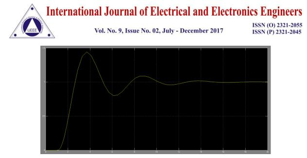
Figure 11: Response With PI Controller
