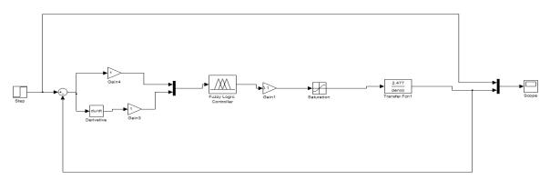
Figure 10: Simulink model with FLC for cruise control
