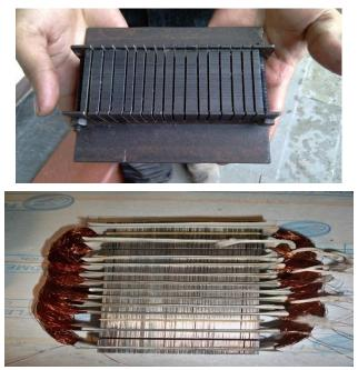
Fig.1.5: Primary stack formation with windings
