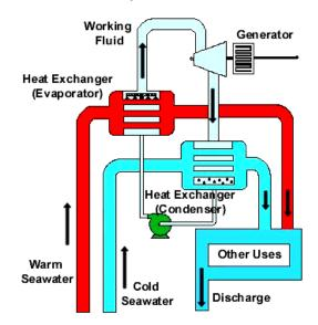
Fig. 2 Schematic diagram of Closed Cycle OTEC [5]
