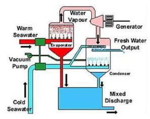
Fig. 1 Schematic diagram of Open Cycle OTEC [5]
