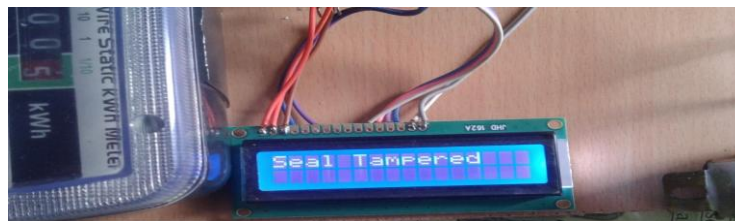
Figure 8 shows tamper happened in energy meter which is displayed on the LCD display.
