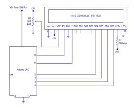
Fig:-4 Speed of the train display
