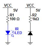
Fig:-2 IR Transmitter and Receiver
