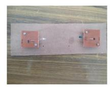
Fig:6 IR transmitter and Receiver
