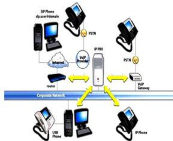
Figure 1: Structure of Voice over Internet Protocol (VOIP)
