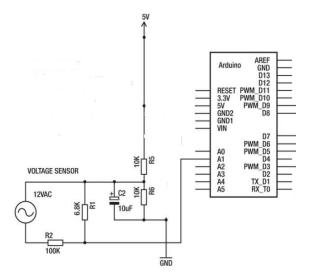
Figure 2: Voltage Sensor
