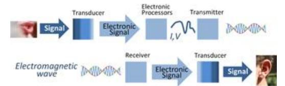
Transducing information such as sound into an electromagnetic pulse signal, which is then sent as an electromagnetic radio wave from a transmitter. A receiver intercepts the radio wave and extracts the information-bearing electronic signal, which is converted back using another transducer such as a speaker.
