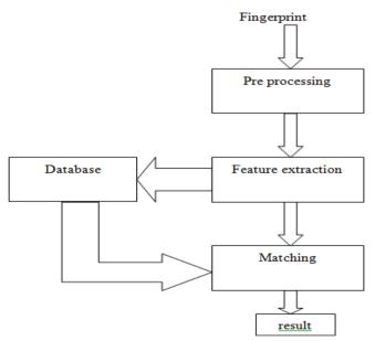
Fingerprint contains ridges and valleys. Fingerprint contain The system will extract the feature and match with database of different orientation fingerprints. different features such as global or local that mean minutiae (ridge ending, ridge bifurcations etc.) The system will extract the feature and match with database.
