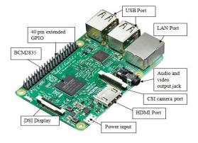
Fig. 1:- Overview of Raspberry Pi Processor
