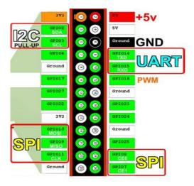
Fig 2:-Overview of GPIO pins
