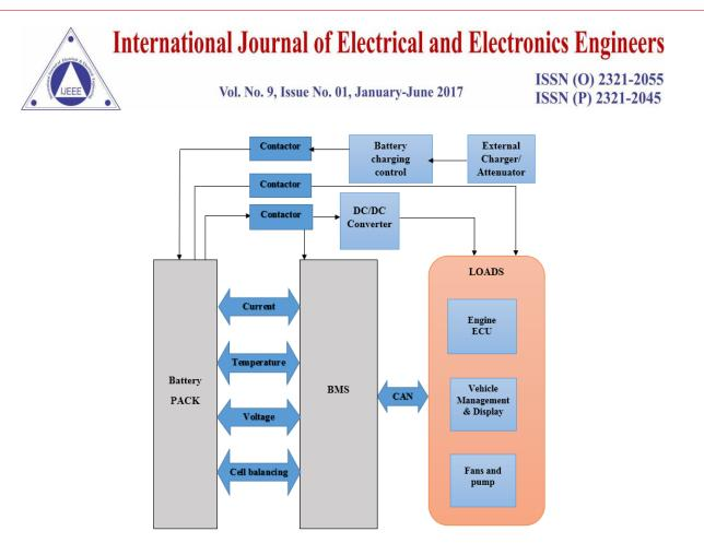
Fig: Basic block diagram of BMS
