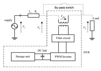
Fig. 1. Typical DVR-connected distribution system.
