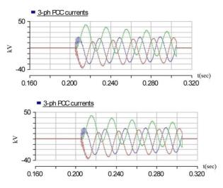
Fig. 13. Current wave shape due to the three-phase short-circuit fault without DVR compensation.
