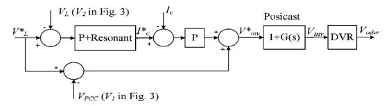
Fig. 5. Multiloop control using the Posicast and P+Resonant controllers.
