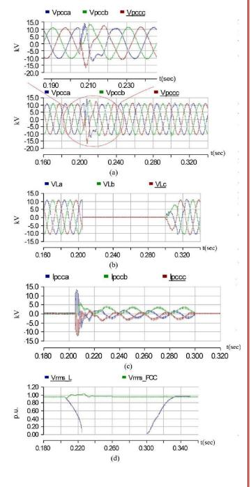
Fig. 11. Starting of an induction motor and the DVR compensation.
