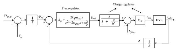
It should also be noted that the reference flux  $(\Phi_{ref})$  is derived by integration of the subtraction of the PCC reference voltage  $(V_*)$  and the DVR load-side voltage. In this control strategy, the control variable used for the outer flux model is the inverter-filtered terminal flux defined as:
