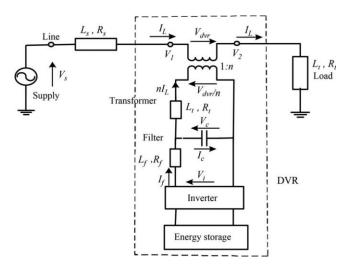
Fig. 3. Distribution system with the DVR.
