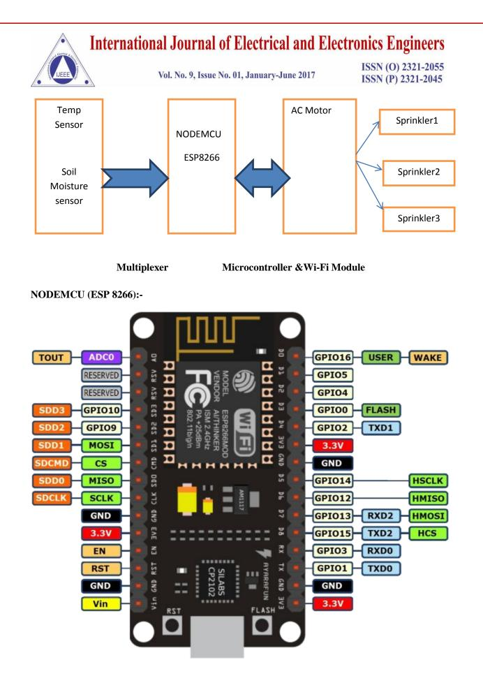
Node MCU is an open-source IOT platform. It includes firmware which runs on the ESP8266 Wi-Fi SOC from expressive systems and hardware which is based on the ESP-12 module. The term NodeMCUby default refers to
