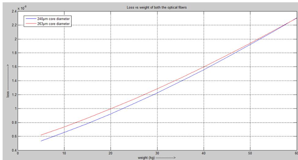
**Figure 7: Loss vs weight comparison curve of different core diameters of optical fibers of 15cm length**
