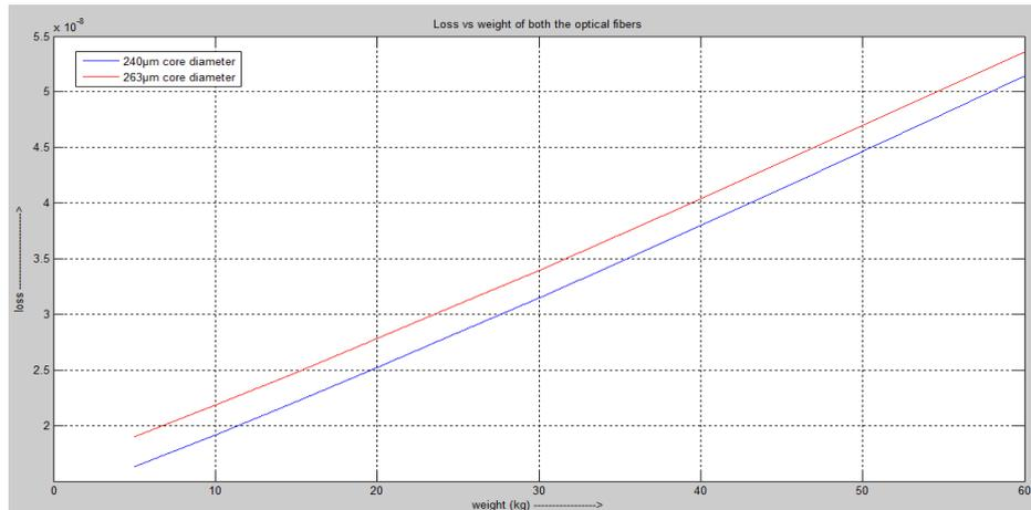
**Figure 9: Loss Vs Weight Comparison Curve of Different Core Diameters of Optical Fibers of 47cm Length**
