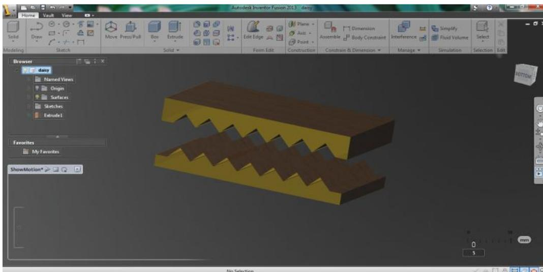
Figure 1: Microbend sensor design in AutoCAD
