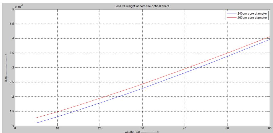
**Figure 8: Loss vs weight comparison curve of different core diameters of optical fibers of 31cm length**
