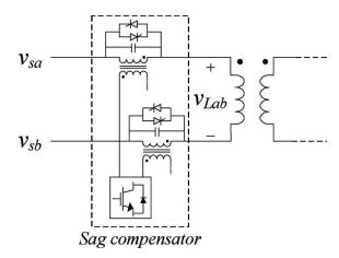
Fig.2 Connection diagram of the proposed system with delta/wye load transformer.
