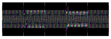
Fig.8 voltage across sensitive load after voltage injection
