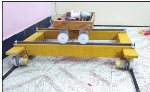
Figure 5.3.1 Hoist model front view
