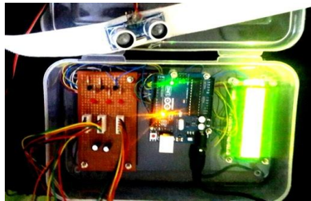
Fig 4: PCB showing Arduino Uno and interfaced components.
