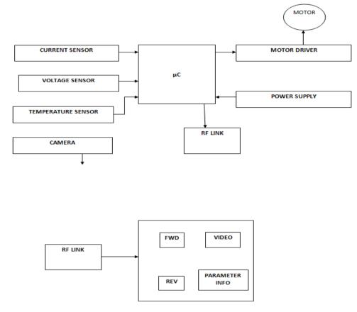
Figure:- Basic Block Diagram of System
