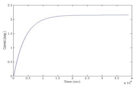
Fig.8. Boost Converter Output Current with P&O Algorithm
