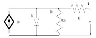
Fig.2. Equivalent Electrical Circuit of a Solar Cell
