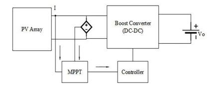
**Fig.1. System Configuration**
