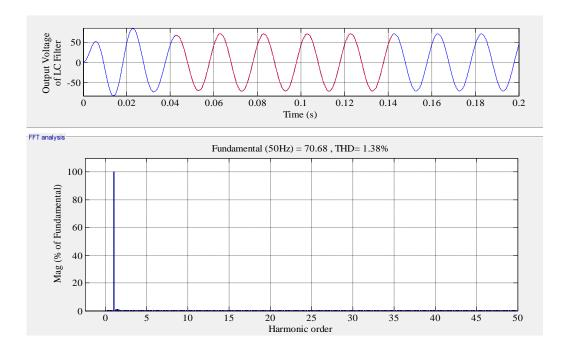
Fig. 13. FFT Analysis of Filter Output Voltage
