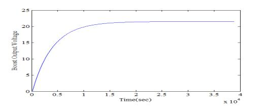
Fig.9. Boost Converter Output Voltage with P&O Algorithm
