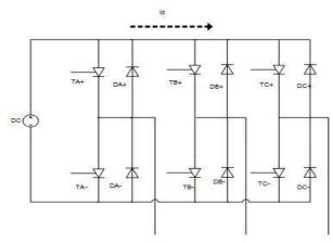
Fig.6. Three Phase Voltage Source Inverter
