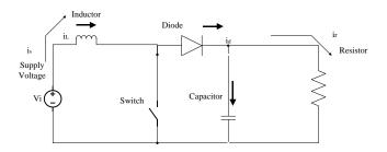
Fig.5. Boost Converter Circuit
