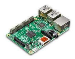
Fig 1: Raspberry Pi Board
