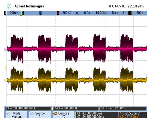
Fig. (6b). Inverter output waveforms CH 1: Sum of Phase Current [1:1] CH 4: Common Mode Current [1:1]
