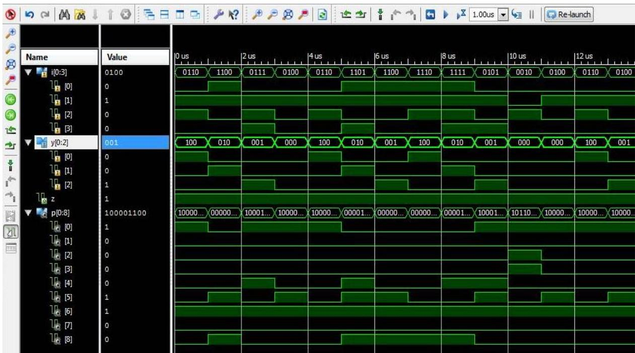
**Figure3. Switching Activity of Skewed Load Tests that are Included in low Power test Set**
