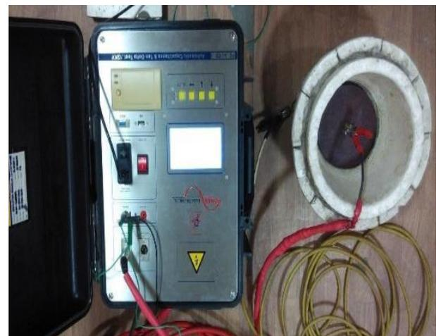
(b) Experimental Test Cell with PE-ACDF-1
