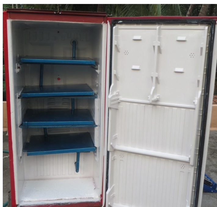
Fig. 15: Drier cabin interior
