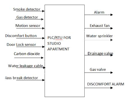
Figure 2.1: The Inputs and Output of the PLC/RTU of the Studio Apartment
