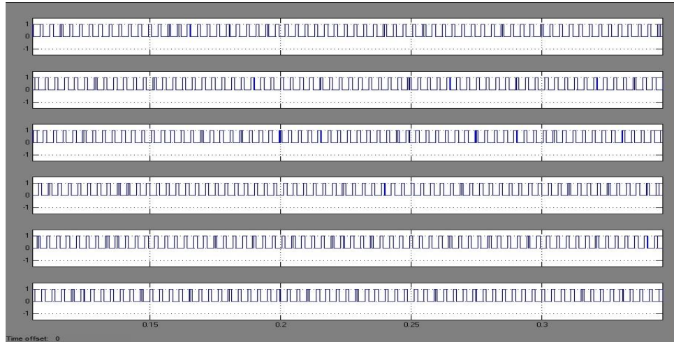
Fig6: switching pulse for Q1 to Q6
