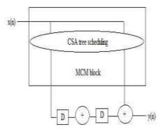
Fig. 3: Tranposed FIR filter
