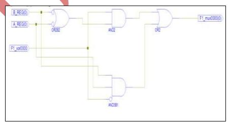
Fig 3.1 Addition Module for Single Bit Addition
