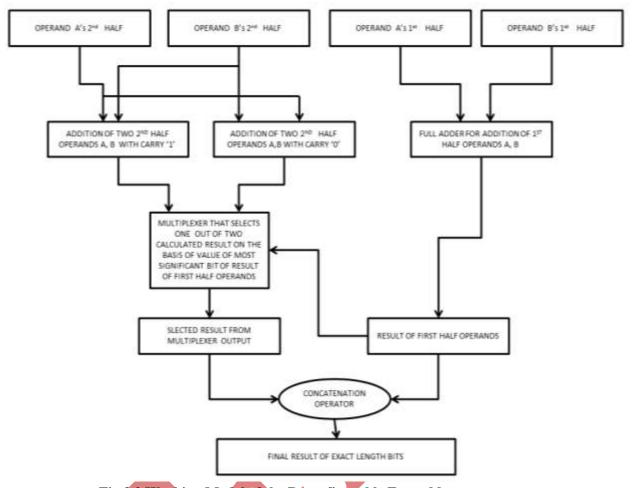
Fig 3.2 Working Model of the Reconfigurable Fast adder
