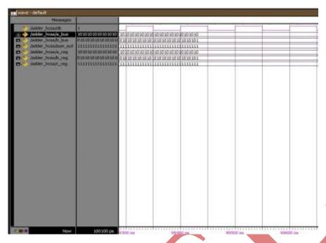
Figure 4.3 Output Waveform for 32 Bit Operands
